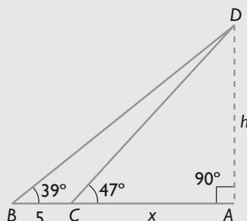
$$\left. \begin{aligned} \text{tg } 47^\circ &= \frac{h}{x} \\ \text{tg } 39^\circ &= \frac{h}{5+x} \end{aligned} \right\} \Rightarrow x = 15,42 \text{ m}$$
