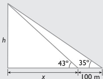
$$\left. \begin{aligned} \operatorname{tg} 43^\circ &= \frac{h}{x} \\ \operatorname{tg} 35^\circ &= \frac{h}{100+x} \end{aligned} \right\} h = 281,07$$
